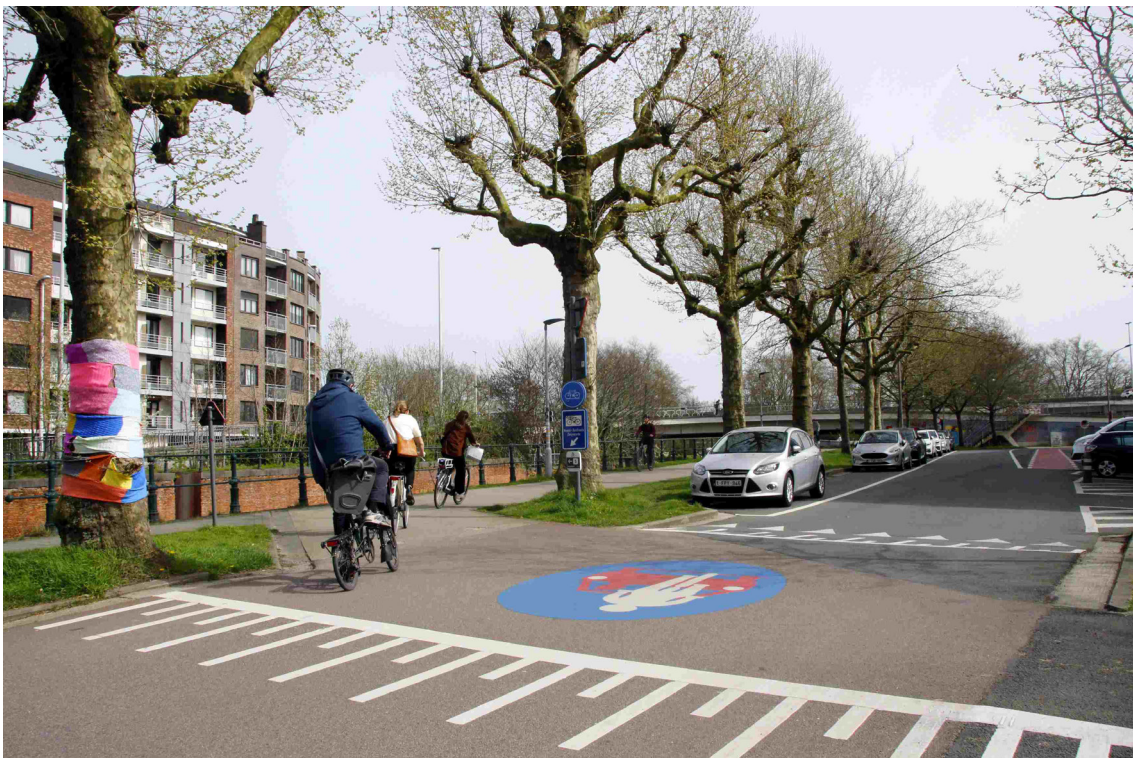
Photo 3 - The speed table on Visserij that leads to the cycle path under the R40
